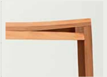
Twin laminations form a curve
